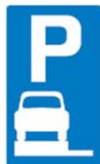
668- vehicles permitted to park wholly on the Footway
